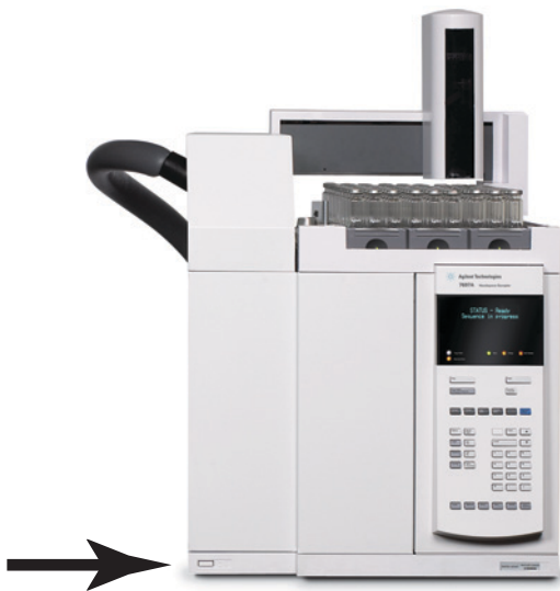
Figure 29 Power on the headspace sampler
