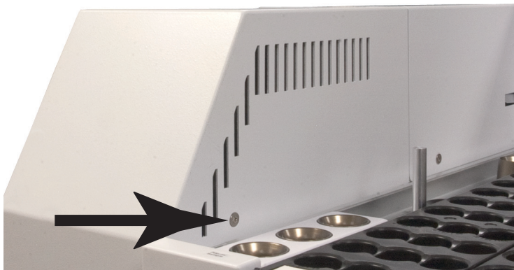
Figure 6 T-20 Torx screw securing the pneumatics front cover
